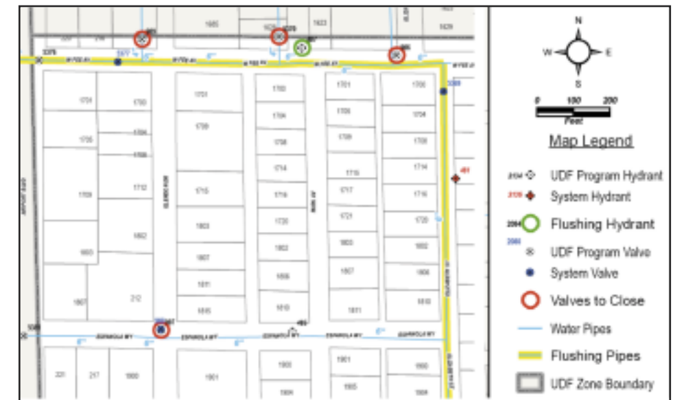
Figure 5: Example of a Typical Valve & Hydrant Map
